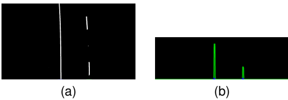
Fig. 7. Example of column histogram operation. (a) Typical input feature map. (b) Column histogram obtained for the Figure 7a.
