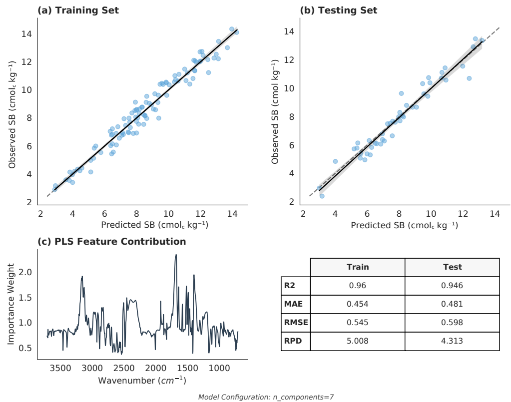
Figure 62 – PLSR results for soil SB prediction based on MIRS spectral data.
