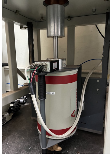
(a) Canberra HPGe GC6020 detector.
