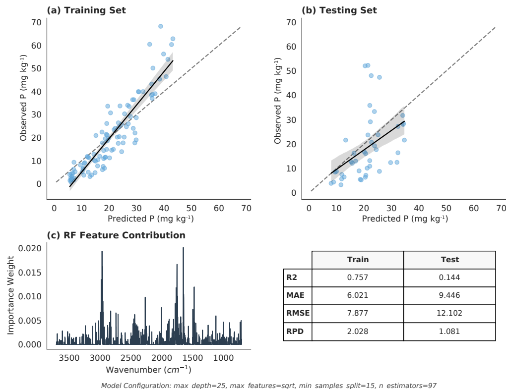
Figure 61 – RFR results for soil exP prediction based on MIRS spectral data.
