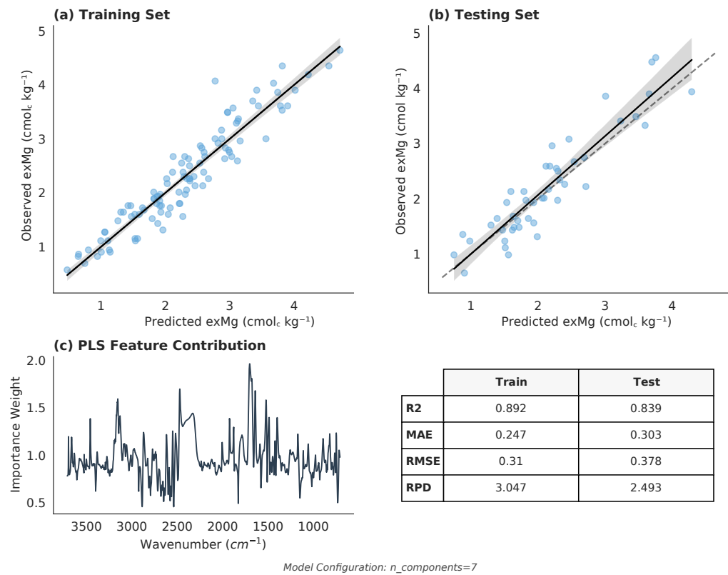
Figure 60 – PLSR results for soil exMg prediction based on MIRS spectral data.
