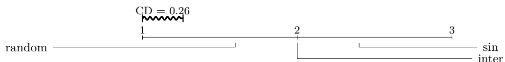
Figure 16 – CD diagram comparing the sinusoidal, intermittent and random attack patterns. The first in the rank corresponds to the greatest RMSE values (best for the attacker).
