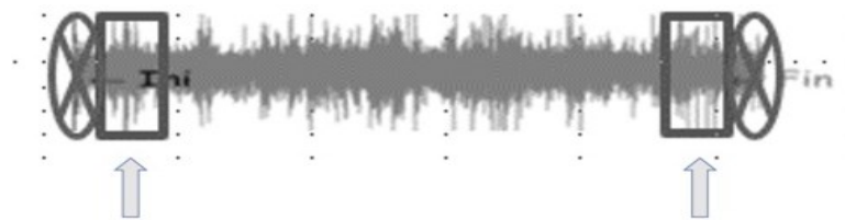
Figure 2. Demonstration of signal processing, with elimination of the initial and final seconds, and then collected the initial and final window.
