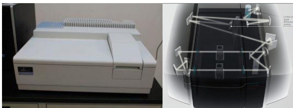
Figura 28 – Espectrofotômetro PerkinElmer UV/Vis Spectrometer Lambda 25 (RENZI, 2015).
