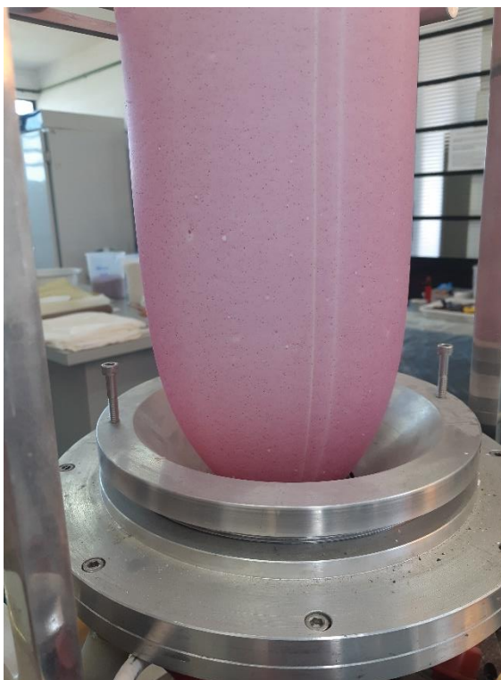
Figure 3 - Extrusion of the multilayer biodegradable film with HP in the active layer ( F_{HP} ).
