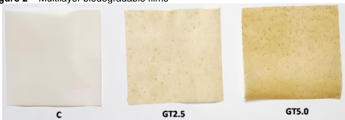
Figure 2 – Multilayer biodegradable films
