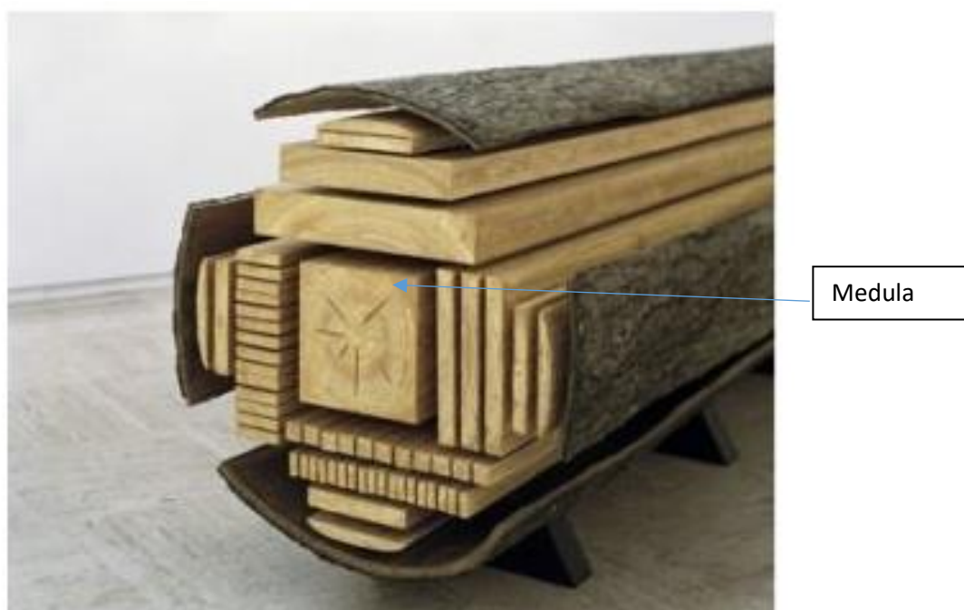
Figura 6 Desdobro da tora de madeira de eucalipto. Fonte: https://www.custom-conference-tables.com/about/case-studies/solid-wood-slab-table-tops-introduction/
