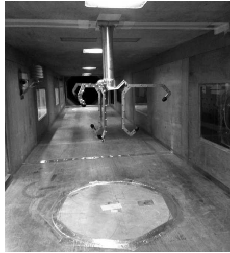
Fig. 8. Experimental arrangement in the wind tunnel used in the tests.
