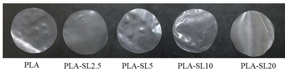
Fig. 1 Visual aspect of the poly(lactic acid)-sophorolipid films PLA, PLA-SL2.5, PLA-SL5, PLA-SL10 and PLA-SL20.
