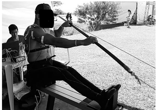
Figure 1 - Parathlete positioned on the ergometer with electromyography signal capture electrodes and heart rate monitor, in the initial position of the sports gesture.
