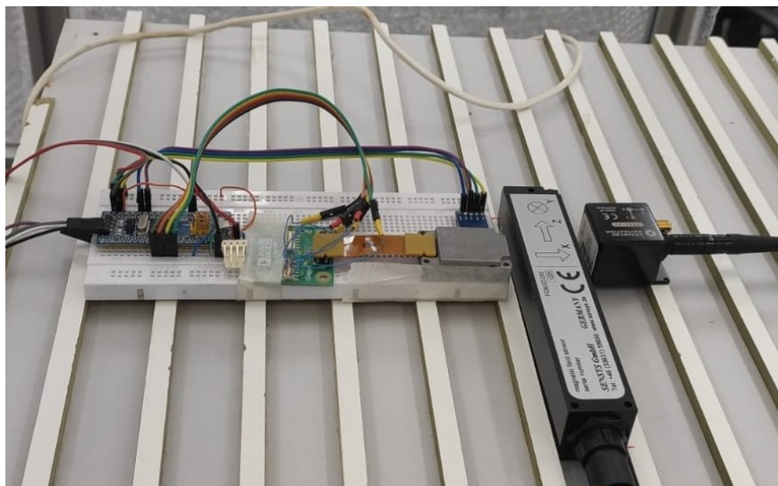
Figure 2.8: Image of the Fluxgate sensor and SUTs during one of the time-varying bias tests.
