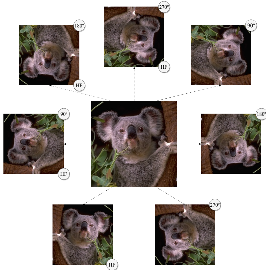
Figure 12 – Process of image augmentation by rotating the original image 3 times and flipping the original and rotated images horizontally.
