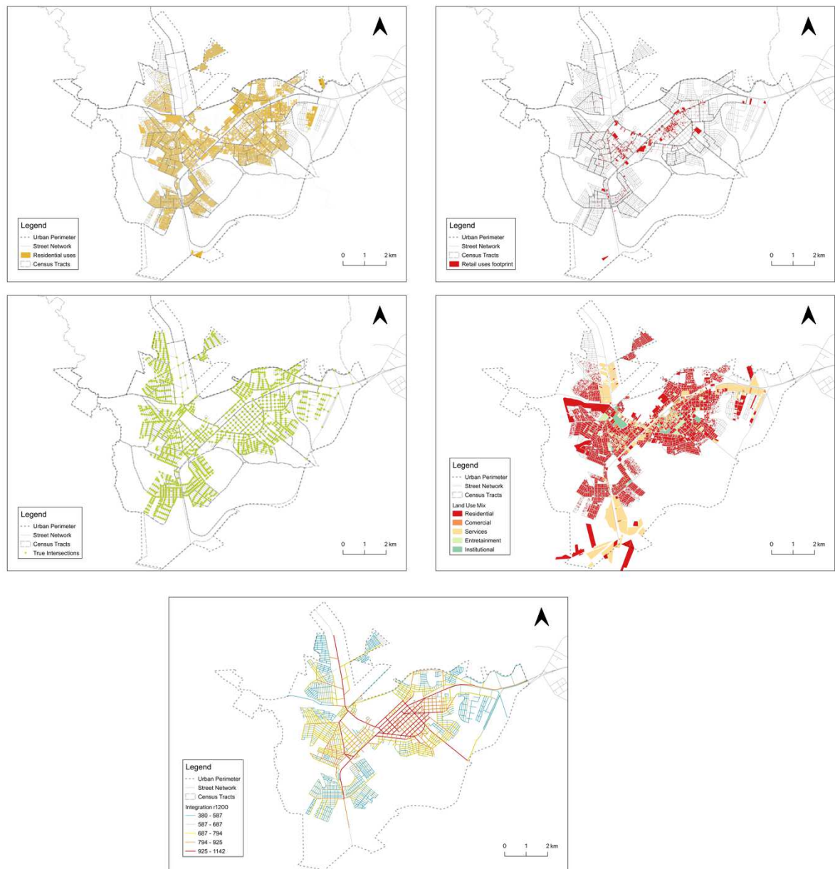
Figure 13 - Macro variable for Rolândia. Respectively: residential parcels, built area (building footprint) for commercial purposes, intersections, land use data, street integration calculations from space syntax.
