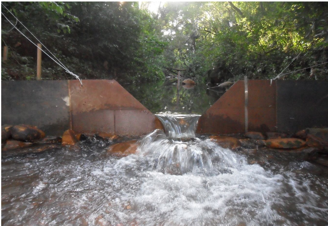
Figura 48 - Vertedouro Triangular Thompson.
