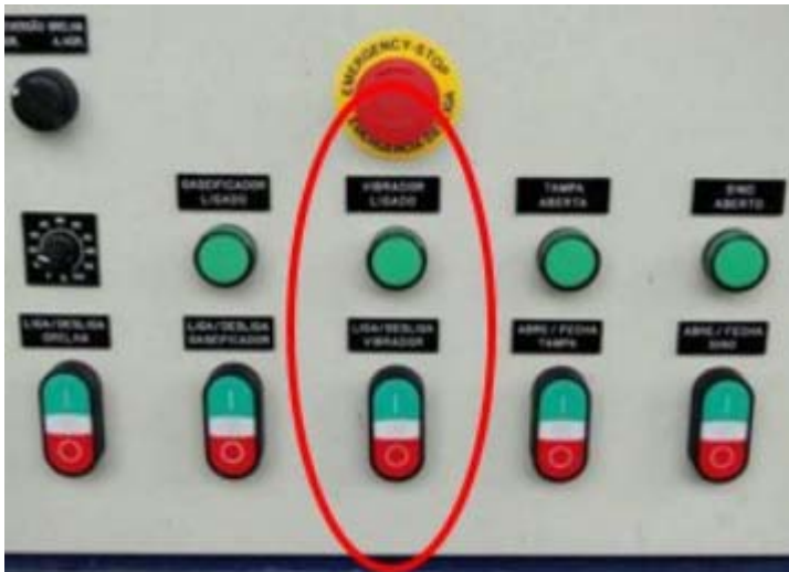
Figura 26 – Botoeira “Liga/Desliga Vibrador”
