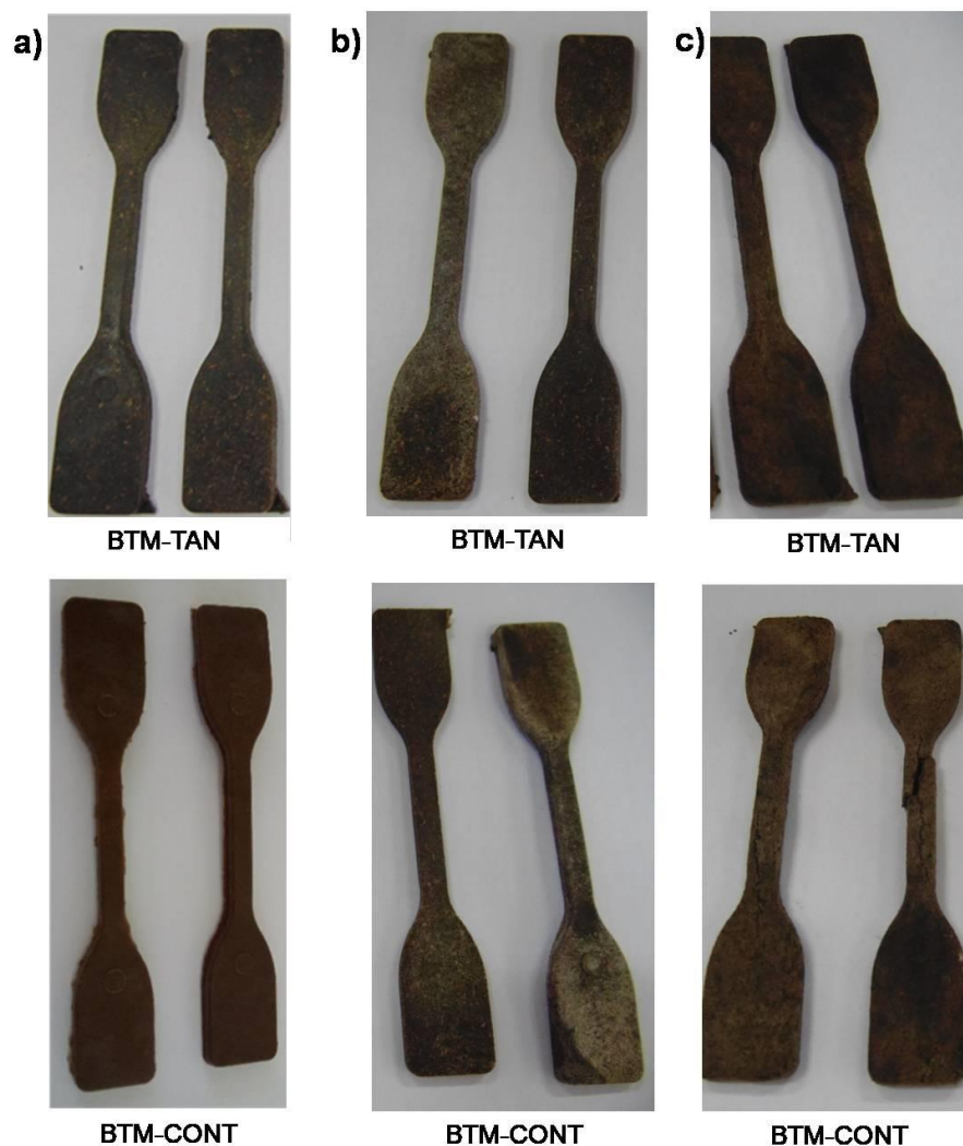
Figure 3. Photographic images of biodegradable thermoset materials (BTM) produced with (BTM-TAN) and without tannin (BTM-CONT) in the formulation before (a) and after 30 (b) or 60 days (c) subjected to biodegradation in a commercial soil substrate recommended for seedlings growth.
