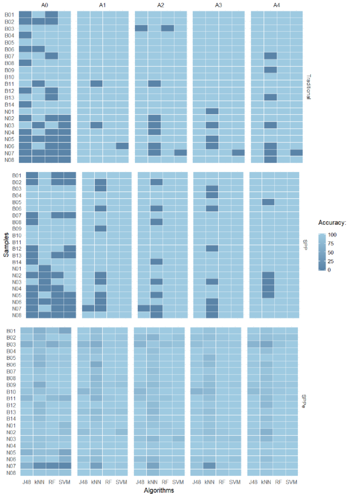
Figure 8 - Accuracy heat map of J48, k-NN, RF, and SVM over the prediction dataset comparing traditional CVS, SPP, and SPPe techniques with repetitions A0, A1, A2, A3, and A4
