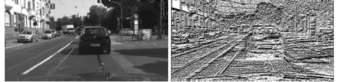
Fig. 1. Sample image from Cityscapes dataset (left) and its corresponding LBP texture map (right).
