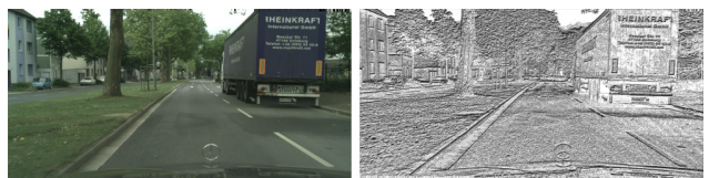
Fig. 1. Sample image from CityScapes [10] dataset (left) and its corresponding LBP texture map (right)
