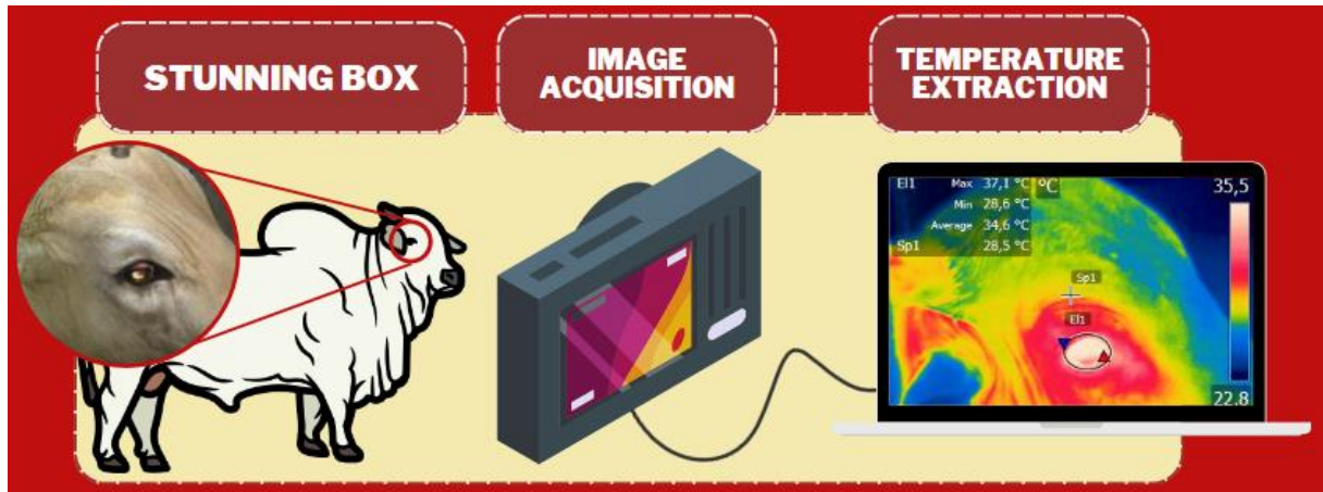
Figure 1. Process of acquiring animals' ocular temperature using infrared thermography in the stunning box at slaughterhouse.
