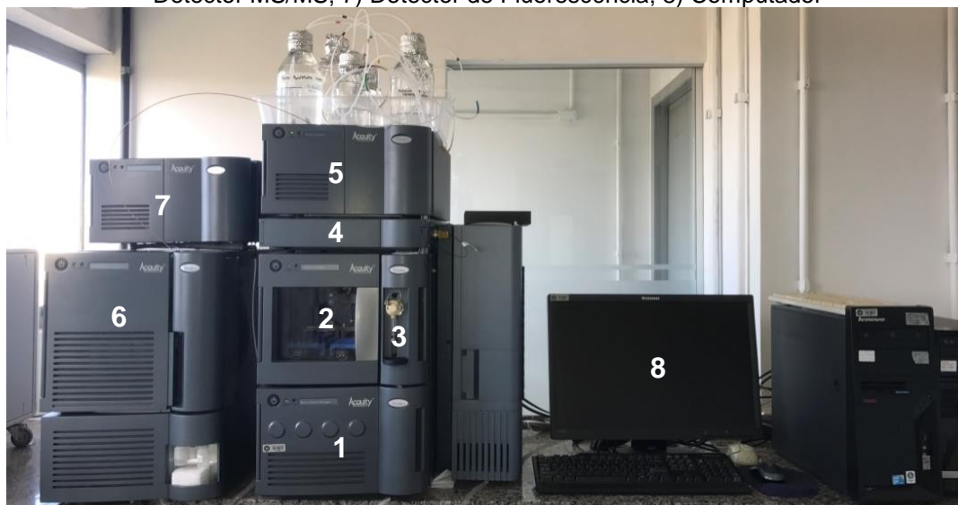
Figura 9 – Módulos do UPLC: 1) Acquity UPLC Binary Solvent Manager (bomba); 2) e 3) Acquity UPLC Sample Manager , amostrador e seringa, respectivamente; 4) Forno; 5) Detector PDA; 6) Detector MS/MS; 7) Detector de Fluorescência; 8) Computador
