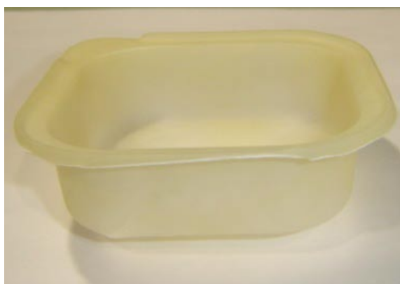
Figure 5. 1. Picture of the object formed in the Labform thermoformer.
