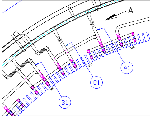
Figure 24 – Detail of couplers installation.
