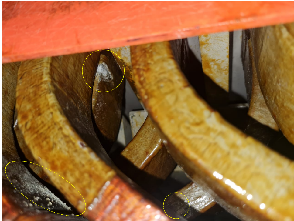
Figure 81 – Corona spots prior to repair, slot 298.
