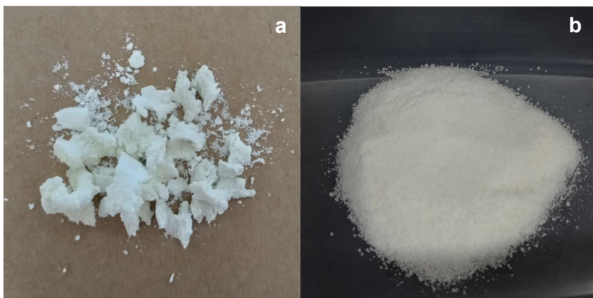
Figure 5.1 – Sample of modified starch obtained through extrusion before (a) and after (b) grinding and sieving.
