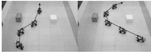
Figure 14. Trajectories described by the robot before (right) and after (left) synaptic learning.
