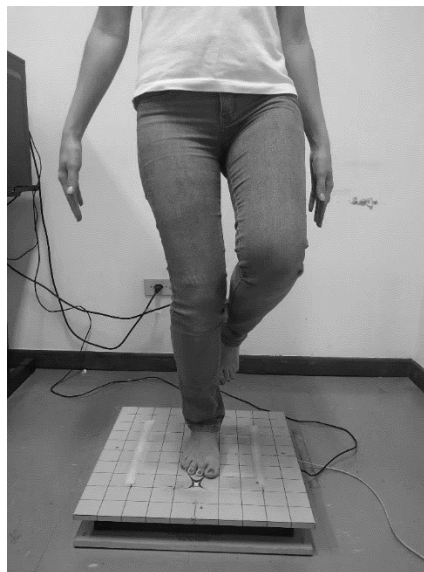
Figure 1: Positioning of the participant on the force platform to collect Postural Control data.
