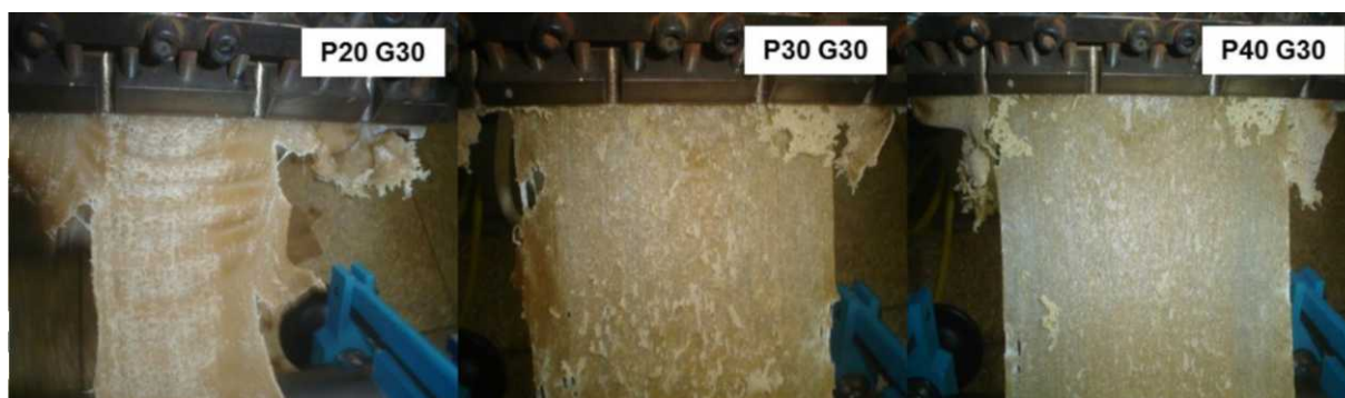
Figure 1 –Biodegradable sheets of PBAT/WOF/GLY at the flat-die exit
