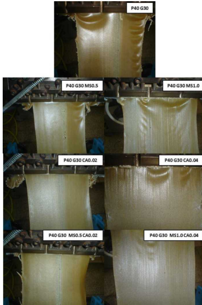
Figure 1 – Biodegradable sheets of PBAT/WOF/GLY/MS/ CA at the flat-die exit
