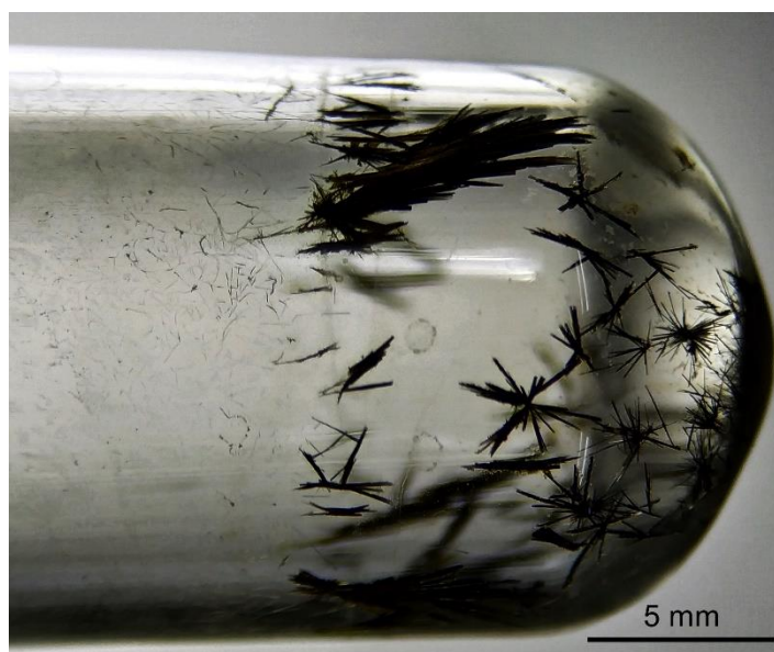
1 Figure 1 - Dark-green thin prismatic crystals of fluopsin C purified from Pseudomonas 2 aeruginosa LV strain supernatant by two sequential flash chromatography processes. 3
